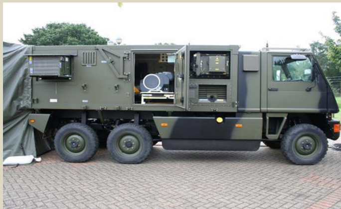
Fig 1. TIGAS with FDG system housed on a MOWAG 6x6 chassis.
